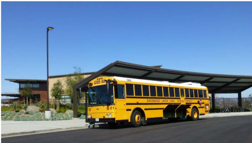
TransPower electric school bus as tested by Escondido Union High School District. The bus uses a Thomas Built Saf-T-Liner HDX school bus. TransPower provides the electric power train.
